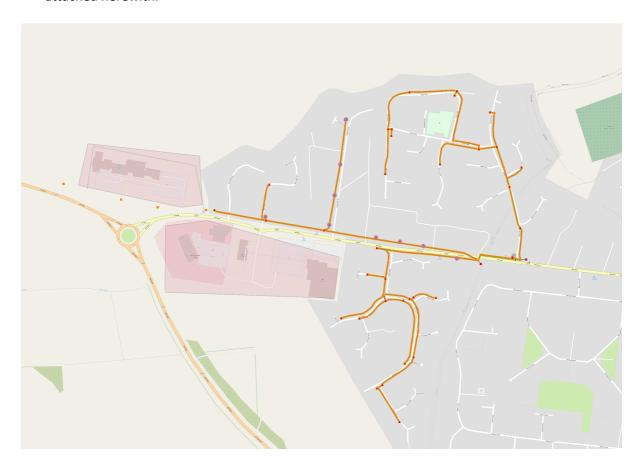
Connexin aims to route fibre cables from the east side to a cabinet located within central Hedon. Subsequently, the distribution cables will leverage KCOM's existing infrastructure, including chambers, poles, and ducts (inventory of which is detailed below).
